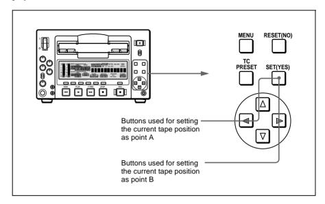
While holding down the SET (YES) button in the menu control section, press the  $\triangleleft$  or  $\triangleright$  button. The time code value of the current tape position is set as point A or B, and a message "A set" or "B set" is displayed for 0.5 second in the time counter display.
